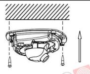
Figure 2-3 Fix the Bottom Board
